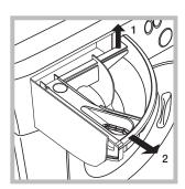
Remove the dispenser by raising it and pulling it out (see figure). Wash it under running water; this operation should be repeated
